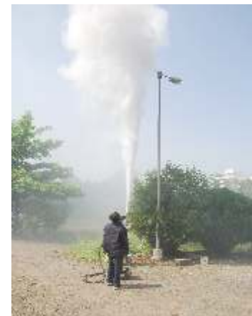
Vertical throw of 10 mtrs shown in reference to 8 mtrs high electric pole
