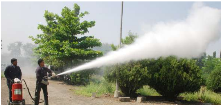
Powder Gun in Action in horizontal as well as vertical throw
